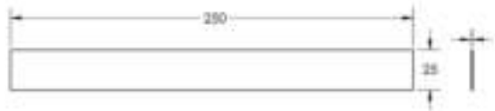
b. Dimension of Tensile Test Specimen of Composite Based on ASTM D3039.
