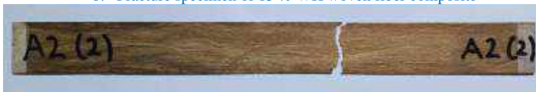
c. Fracture specimen of 25 % unidirectional WH fiber composite
