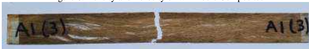
a. Fracture specimen of 15 % unidirectional WH fiber composite.
