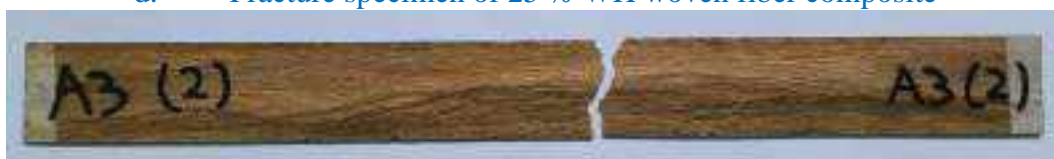
e. Fracture specimen of 35 % unidirectional WH fiber composite
