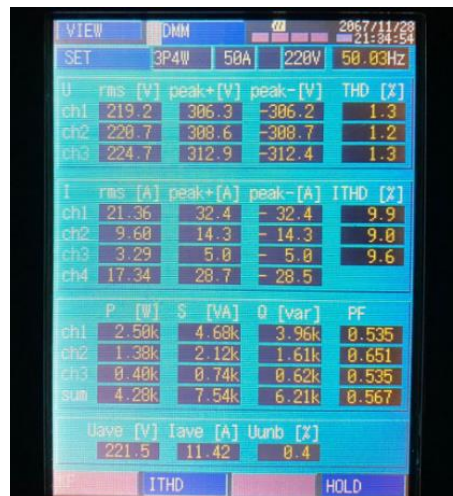
Figure 2. Measurement result of power quality parameter on the 3 rd floor SDP panel.
