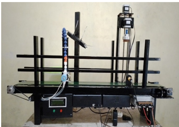
Figure 3. Prototype of an automatic drinking water filling device.
