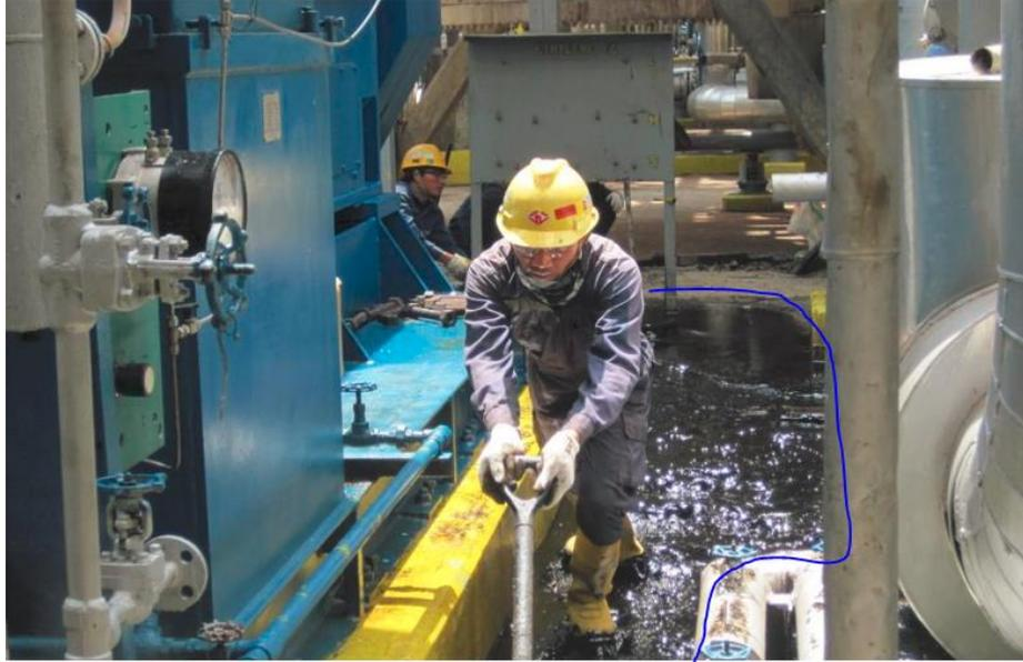
**Gambar 4.22** Environment Issue karena Tumpahan Quench Oil Langsung ke Tanah
