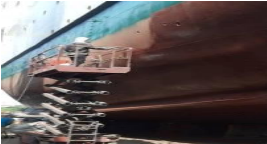
Gambar. 5 Kegiatan Anti Fouling Coating Process KMP. Doro Londa
