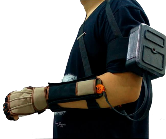
Fig. 1. Fabric-based soft exoskeleton glove (a) Soft glove system (b) Portable soft glove when worn by a user.
