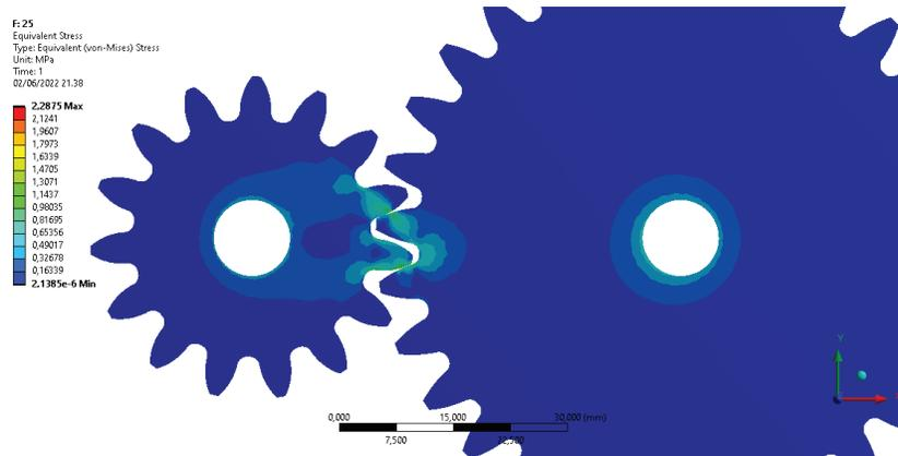
**FIGURE 5.** Von Mises Contour of the Optimized Plastic Gear.
