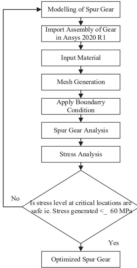
FIGURE 3. Flowchart of shape optimization plastic gear
